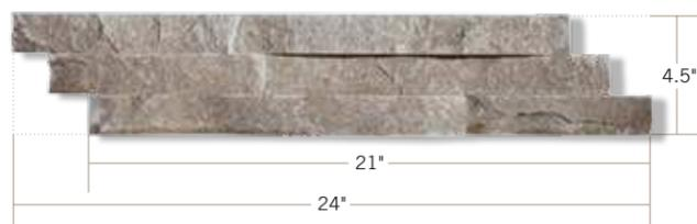
**European Ledge** creates a perfect fusion of old-world stonework and modern design. The 1.5" precision-cut ledge stones are molded into 4.5" h x 24" w panels. The stair stepped edge creates a tight-fit, eliminating unsightly vertical joints.
