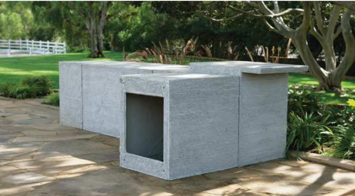
**THE BUILDING BLOCKS.** Eldorado Outdoor products quickly assemble into a virtually limitless combination of configurations. Each piece is made of glass-fiber reinforced concrete (GFRC) which can be installed on any solid flooring surface without concrete footings or rebar.
